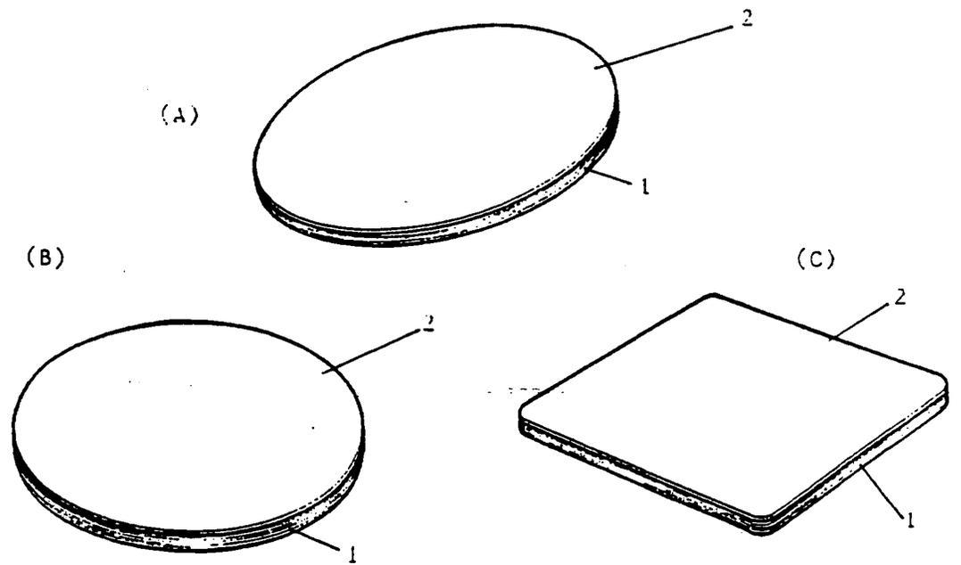
Tissue sheet with degradable impermeable layer - comprises impermeable film layer made of coating of colloidal substance e.g. gelatin, or moisture-resistant resin e.g. amide; EPICHLOROHYDRIN DEXTRIN
